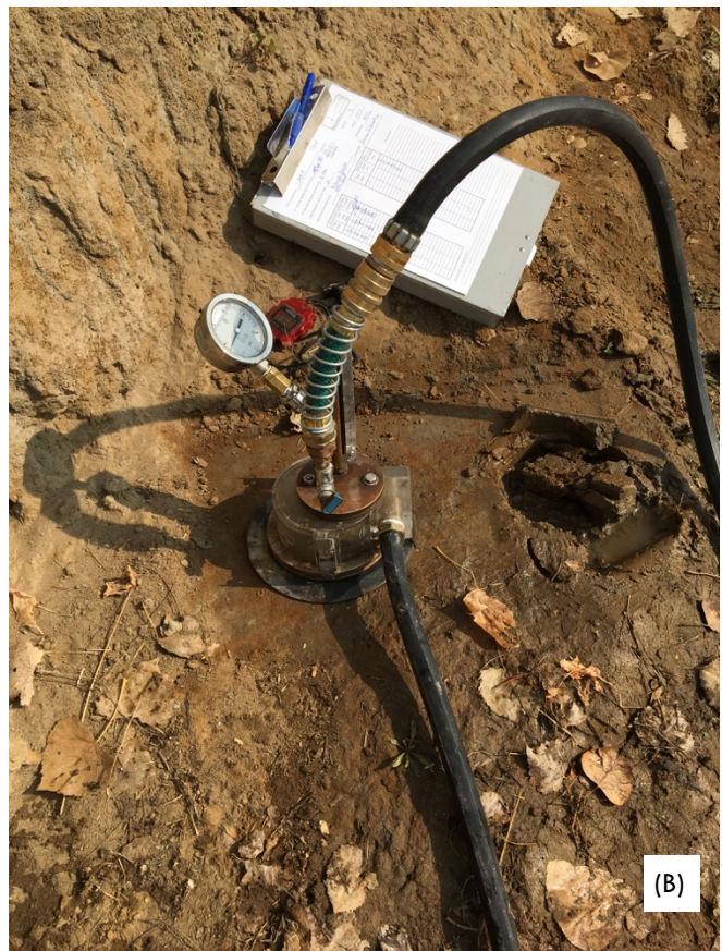
FIGURE 34 – PHOTOS OF THE LOWER BANK SOIL AT STUDY SITE LAR9 ON THE AMERICAN RIVER ON WHICH JETS WERE CONDUCTED: (A) ABOUT 2 M ABOVE WATER LINE, AND (B) NEAR THE WATER LINE.
