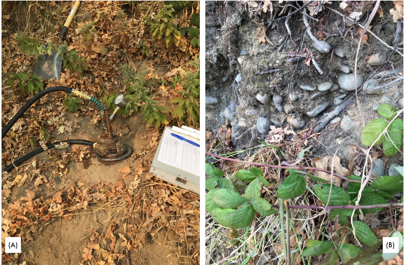
FIGURE 11 – PHOTOS OF BANK SOILS AT STUDY SITE LAR2 ON THE AMERICAN RIVER: (A) SANDY SOIL AT JET LOCATION AND (B) SANDY GRAVEL AT BANK TOE.
